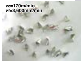
Well-shape chips by high-feed boring.
